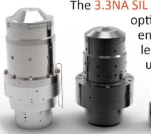
The 3.3NA SIL objective is the latest in our family of custom designed lenses optimized to provide superior, diffraction-limited imaging over the entire field-of-view. Our patented self-aligning SIL tip automatically levels to conform to the local contour of the device under test. Our unique tip flexure design provides the lowest contact force in the industry, so it is suitable for imaging mounted devices or
